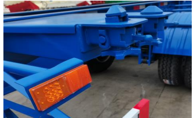
Durable and Liftable container lock Optional to install 8 or 12 container locks
